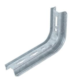
TP support/bracket for fastening to horizontal concrete ceilings and walls. If the profile is fastened directly to the ceiling or the profile is screwed together as head reinforcement, then, for reasons of stability, always use the spacer, type DS
