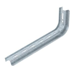
TP support/bracket for fastening to horizontal concrete ceilings and walls. If the profile is fastened directly to the ceiling or the profile is screwed together as head reinforcement, then, for reasons of stability, always use the spacer, type DS
