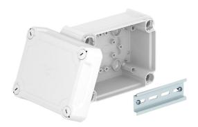
Closed junction box for the connection of cables in indoor and protected outdoor areas. Rectangular design without entries. Suitable for wall and ceiling mounting and on mounting panels. With the option of fastening inside and to mount via the corner domes. High cover with quick lock, sealable. Made from halogen-free and UV-resistant materials.
