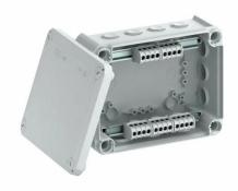
Junction box with terminal strip for the connection of cables and lines indoors and in protected outdoor areas. Rectangular design with plug-in seals to the sides and knock-out entries in the bottom. Suitable for wall and ceiling mounting and on mounting panels. With the option to fasten inside and to mount via the corner domes. Cover with quick lock, sealable. Made from halogen-free and UVresistant materials.
