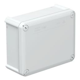
Junction box for the connection of cables and lines indoors and in protected outdoor areas. Rectangular design without entries. Suitable for wall and ceiling mounting and on mounting panels. With the option to fasten inside and to mount via the corner domes. Cover with quick lock, sealable. Made from halogen-free and UV-resistant materials.
