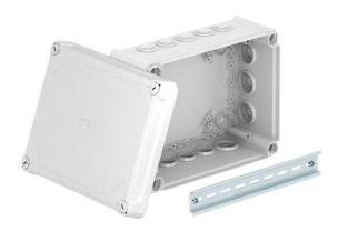
Junction box for the connection of cables and lines indoors and in protected outdoor areas. Rectangular design with plug-in seals to the sides and knock-out entries in the bottom. Suitable for wall and ceiling mounting, on mounting panels and threads in the floor. With the option to fasten inside and to mount via the corner domes. High, transparent cover with quick lock, sealable. Made from halogen-free and UV-resistant materials.
