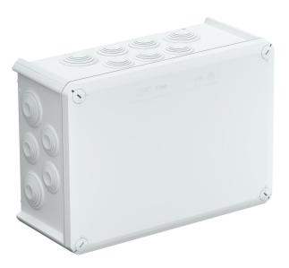
Junction box for the connection of cables and lines indoors and in protected outdoor areas. Rectangular design with plug-in seals to the sides and knock-out entries in the bottom. Suitable for wall and ceiling mounting and on mounting panels. With the option to fasten inside and to mount via the corner domes. Cover with quick lock, sealable. Made from halogen-free materials. Flame-resistant type made from special polypropylene.
