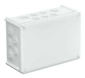
Junction box for the connection of cables and lines indoors and in protected outdoor areas. Rectangular design with plug-in seals to the sides and knock-out entries in the bottom. Suitable for wall and ceiling mounting and on mounting panels. With the option to fasten inside and to mount via the corner domes. Cover with quick lock, sealable. Made from halogen-free and UV-resistant materials.
