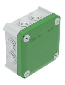
Junction box for the connection of cables indoors and in protected outdoor areas. Square design with plug-in seals to the sides and knock-out entries in the bottom. Suitable for wall and ceiling mounting and on mounting panels. With the option of fastening inside and to mount via the corner domes. Green cover for the labelling of specially designated cables and special circuits in the electrical installation (e.g. backup power, bus systems, etc.). Cover with quick lock, sealable.
