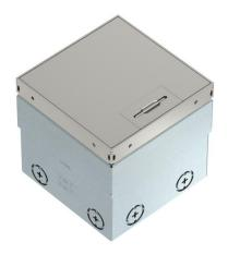
Square floor socket for use in dry-care cavity and screed floors in indoor areas. Installation housing with pre-marked insertion openings for pipes (M20/M25). Cover adjustable to top edge of floor covering using four height-adjustment supports. The minimum installation depth is 100 mm, the height-adjustment range is +35 mm.
