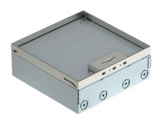
Square floor box for use in dry-cleaned cavity and screed floors for indoor use. Installation housing with pre-marked insertion openings for pipes (M25). Cover adjustable to top edge of floor covering using four height-adjustment supports. 15 mm floor covering recess in the hinged cover. The minimum installation depth is 95 mm, the height-adjustment range + 30 mm.
