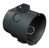
Device/connection socket with torsion-resistant guaranteed standard combination spacing of 71 mm (to DIN 49 073-1) through Snap–lock coupling. Break-out openings for cables and pipes Ø 20 mm and Ø 25 mm. Combinable for spreading and screw fastening, low-lying plaster brackets, device bolt spacing 60 mm, for screw fastening with 3.2 mm self-tapping screws, with 2 screw bosses without screws, protection rating IP20.
