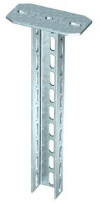
U support in fixed lengths. Dimensions 70 x 50 mm. In the case of bracket mounting on both sides, or when mounting the bracket at the end of the support, use the spacer of type DSK 61. The surface coating is a coating created in a single-dip method with extra-high zinc thicknesses.
