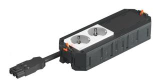
The ready-for-connection UTC4 universal support has 2 pre-installed 33° protective contact sockets in white and 2 blanking covers for retroinstallation of 2 installation devices of the Modul 45 series. Suitable for VL connection cables and device installation units of nominal size R7, R9 and 9.
