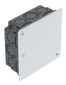
Flush-mounted connection box for clamping terminals, for use in masonry with an installation depth of at least 45 mm. With cover and cover screws (15 mm). Flat cover edge, roughened surface.
