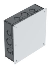
Flush-mounted connection box for clamping terminals, for use in masonry with an installation depth of at least 65 mm. With cover and cover screws (15 mm). Flat cover edge, roughened surface.
