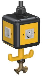
Housing equipped and prewired, with 1 m pipe 1/2" and connection for compressed air hose 13 x 3.5 mm and 2-way distributor 1/2", with suspension lug, grip hook and four cover plates.
