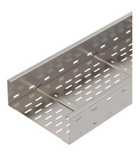
Wide span cable tray system, perforated, with a side height of 110 mm. Straight connectors of type WRVL 110 should be ordered separately and in the appropriate quantity.
