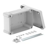
Junction box with hat profile rail for the connection of cables and lines indoors and in outdoor areas. Rectangular design without entries. Suitable for wall and ceiling mounting with the option to fasten outside, inside or to mount via the corner domes. Particularly impact resistant with IK09. Cover with quick lock, sealable. Made from halogen-free and UV-resistant materials.
