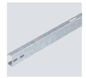
Support profile to mount photovoltaic modules on free-standing systems. Mounting of support profile on pre-mounted supports with KV FT cross-connectors. Mounting of the PV modules on the support profile with end and/or connection clamps. Connection of multiple support profiles with LV FT straight connectors and KV FT cross-connectors, screw-on.
