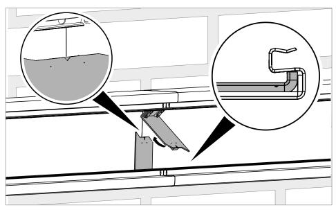
Fig. 28: Inserting the side sections of the connector set
