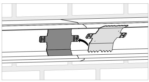
Fig. 30: Mounting connector PLM 0404
