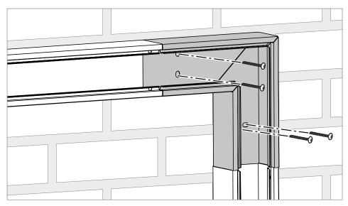
Fig. 14: Mounting fitting
