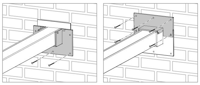
Fig. 47: Mounting the wall connection collar
