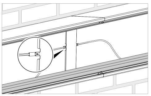
Fig. 31: Attaching the protective conductor
