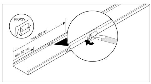
Fig. 33: Inserting locking brackets in the duct cover
