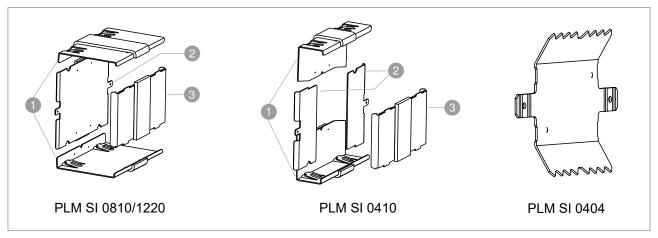
Fig. 25: Joint connector PLM SI...
