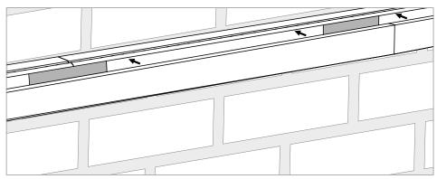
Fig. 36: Snapping-in the duct cover offset
