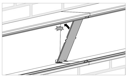
Fig. 27: Inserting the floor plate
