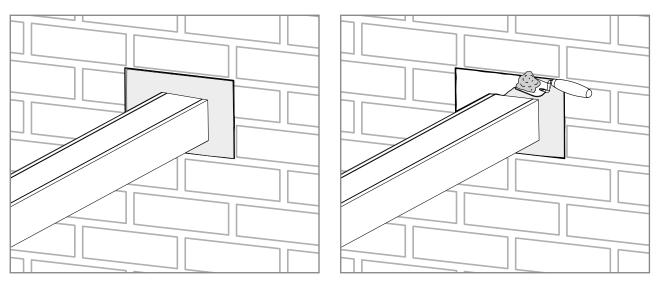
Fig. 46: Sealing the remaining opening
