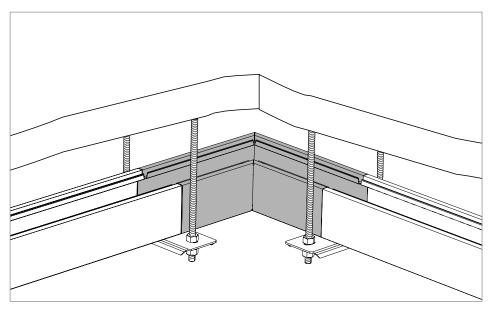
Fig. 18: Mounting fittings on supports
