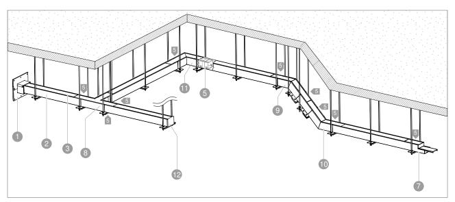
Fig. 2: System overview for suspended mounting
