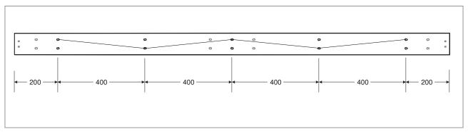
Fig. 6: Hole pattern for vertical wall and ceiling mounting
