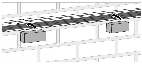
Fig. 35: Inserting the foam cable outlet
