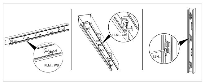
Fig. 8: Mounting the duct trough
