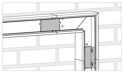
Fig. 15: Mounting joint connectors
