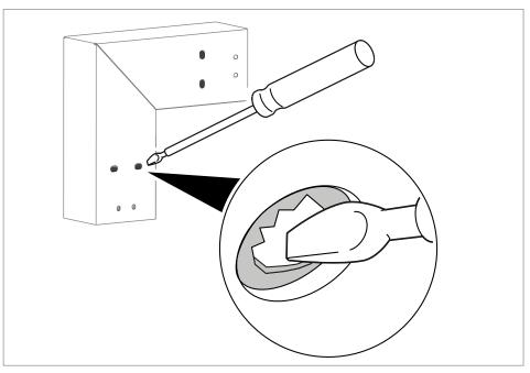
Fig. 21: Piercing the fire protection fabric at the fastening points
