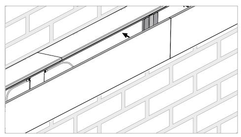
Fig. 34: Snapping-in the duct cover offset
