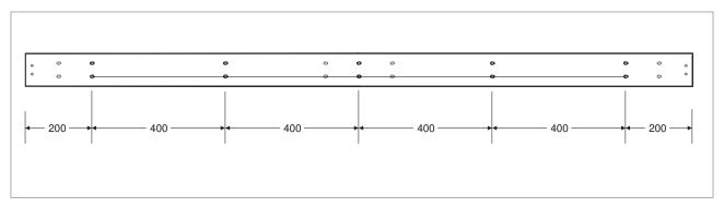
Fig. 5: Hole pattern for horizontal wall mounting
