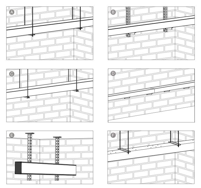
Fig. 4: Overview of mounting on support systems
