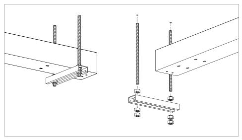
Fig. 20: Mounting support system for fitting
