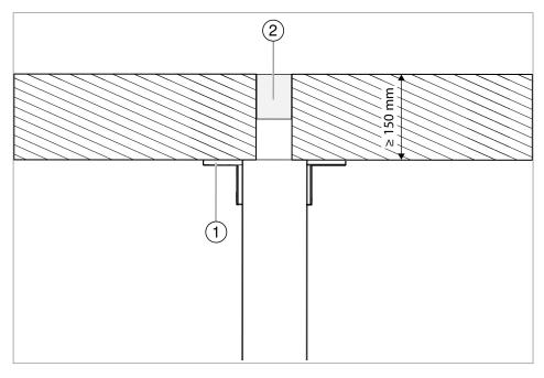
Fig. 48: Ceiling connector El30-El90
