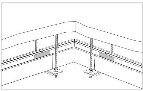
Fig. 19: Mounting the joint connectors
