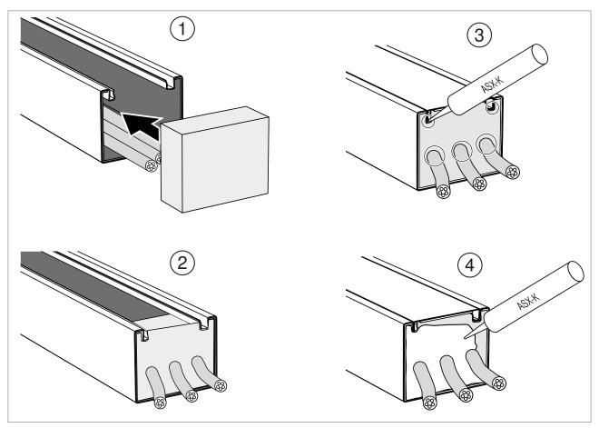
Fig. 38: Multiple cable outlet
