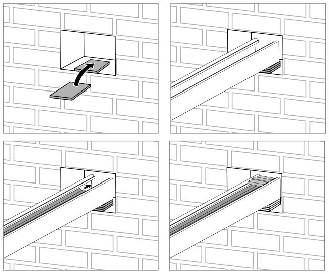
Fig. 45: Installing ducts
