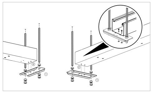
Fig. 16: Mounting the suspension at the joint
