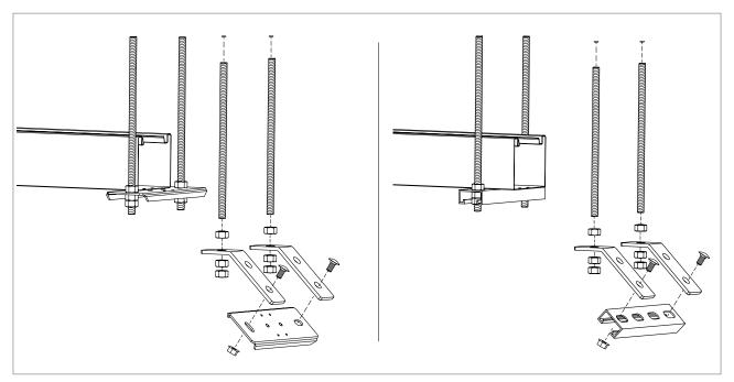
Fig. 23: Mounting the mounting angle
