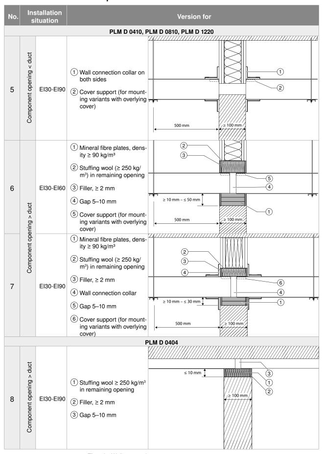
Fig. 42: Wall penetration
