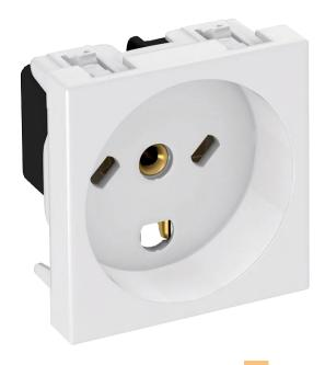
Socket, single 0°, to Danish standard, encoded for IT power circuit, with screw terminals, 2-pin, 16 A 250 V  $^\sim$  , with connection terminals to IEC 60884-1.
