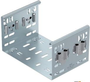
Magic straight connector for direct and screwless joining of Magic fittings with a side height of
