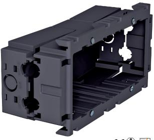
Front locking accessory mounting box for standard switch ranges for the installation of two individual installation devices or a multiple protective contact socket. With unfolding, and also removable, base for time-saving cable connection and with feed openings for cable diameters of up to 14 mm. Halogen-free version.
