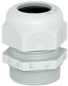
The quickest and most convenient way of providing strain relief and tightness with cable glands on junction boxes and housings is with the tried-and-trusted V-TEC VM cable glands from OBO. A protection rating of IP68 is achieved through the integrated sealing lip and the special OBO slat  $\,$ technology. Strain relief and tightness have been tested to DIN EN 62444.
